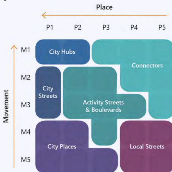
Figure 3.5. Australia’s Movement and Place Framework
